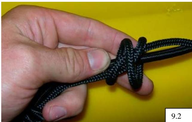
3. Working to the left of the previous knot, begin the second half of knot #1 by taking the bungee and looping it over the retract line two times, from right to left in a
