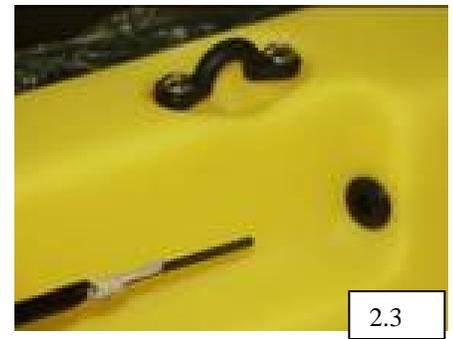
6. Reach inside the stern access hole to pull the tubing through the hull and guide it through the stern grommet. Hold your fingers over the grommet as you pull the tubing through so the grommet stays in place. Remove the wire. See 2.4
