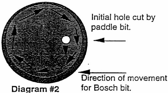
3. Insert the router in the hole and move toward the edge in a clockwise direction.
