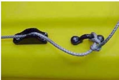
1. The rudder retraction line should go through the center of the rudder housing. Continue pulling the line up toward the seat and through the loop in the hatch/gear straps along the right side of the kayak to keep the line out of the way.
