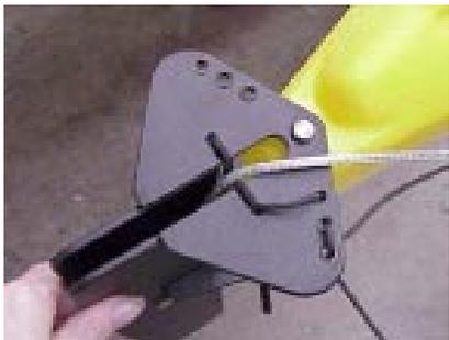
1. At the stern of the kayak, put the end of each steering line down through the top of the shoulder washer in the middle hole on each side of the rudder steering plate.
