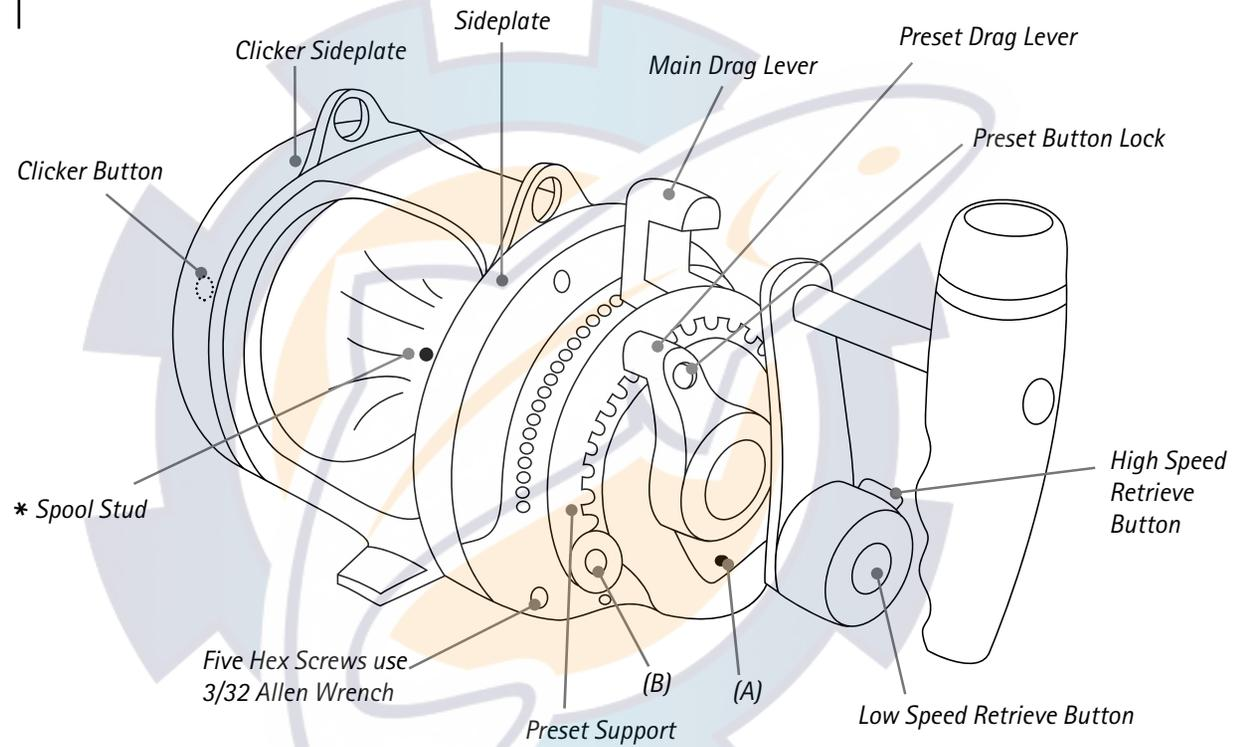
\* The spool stud for tying the line to the reel can be removed with a phillips screwdriver.
