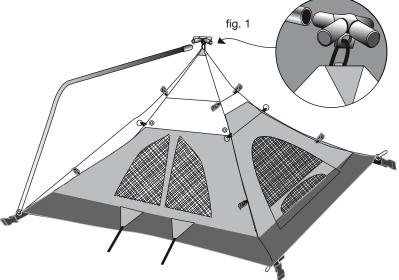
4. Insert the next pole onto the opposite arm on the spider. Tension this assembly by placing the corner pin in the other end of this pole. See fig.2.
