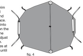
8. Stake out the tent through the corner rings. Stake opposite corners while applying tension to square the tent and remove wrinkles from the floor. Stake out the fly through the rings on the side of the fly. Stake down the side pull outs to provide maximum floor space. See fig.5.
